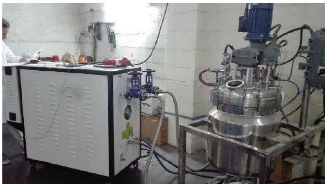
COLOR CENTER – pilot capacity: 65 kg TEXAFOB ARK (paraffin-based DWR product)
