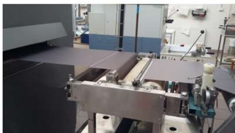
R2R Werner-Mathis continuous line (INOTEX), width 45 cm (INOTEX), strips 3 - 3,2 m
